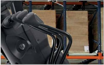
**Optional Fingertip Controls** – These controls are mounted to the armrest and allow the operator to easily manipulate the hydraulic system from a comfortable position.
